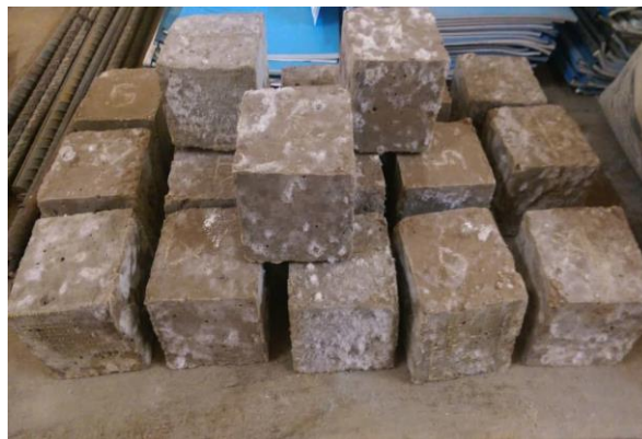
Plate 3.1: Geopolymer Mortar Cubes
