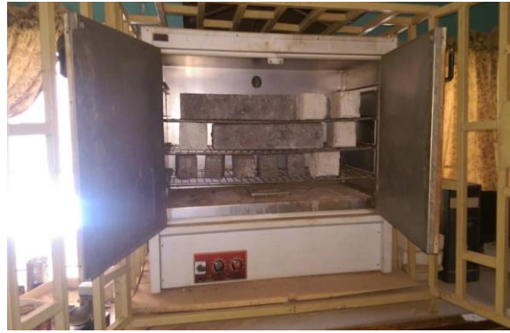
Plate 2.1: Oven Curing of Geopolymer Specimens
